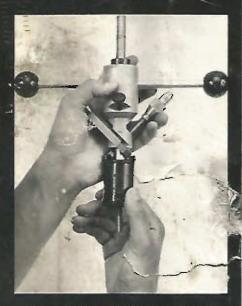
Install the pilot in the tool and insert calibrating gauge on the pilot with the desired angle (30° to 45°) on the gauge facing the cutters.
