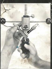
Feed 60° cutter on tool downward until it touches the calibrator.
