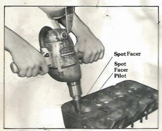
1. Spot facing is only required for integral valve guides. Select proper spot facer pilot. Install spot facer pilot and spot facer in drill. Spot face top of valve guide to assure that the cutter pilot will fit squarely against it.
