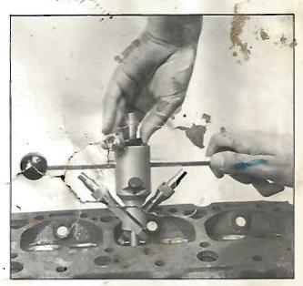
10. To remove tool, loosen feed nut locking screw. Turn tool clockwise and turn feed nut counter clockwise until cutters are clear of seat.
