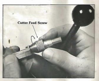
4. Set micrometer cutter adjustment to measurement of valve diameter. Always turn cutter feed screw in a clockwise direction when making the final cutter setting. This should be done on both cutters. Retighten cutter locking screws.
